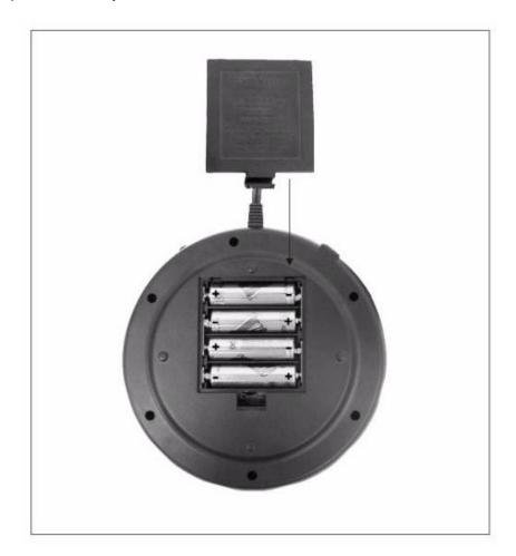
Note: When batteries begin to lose their charge, the system will automatically run low power detection. Thus, a battery symbol will appear on the TV screen to indicate to change the batteries.
